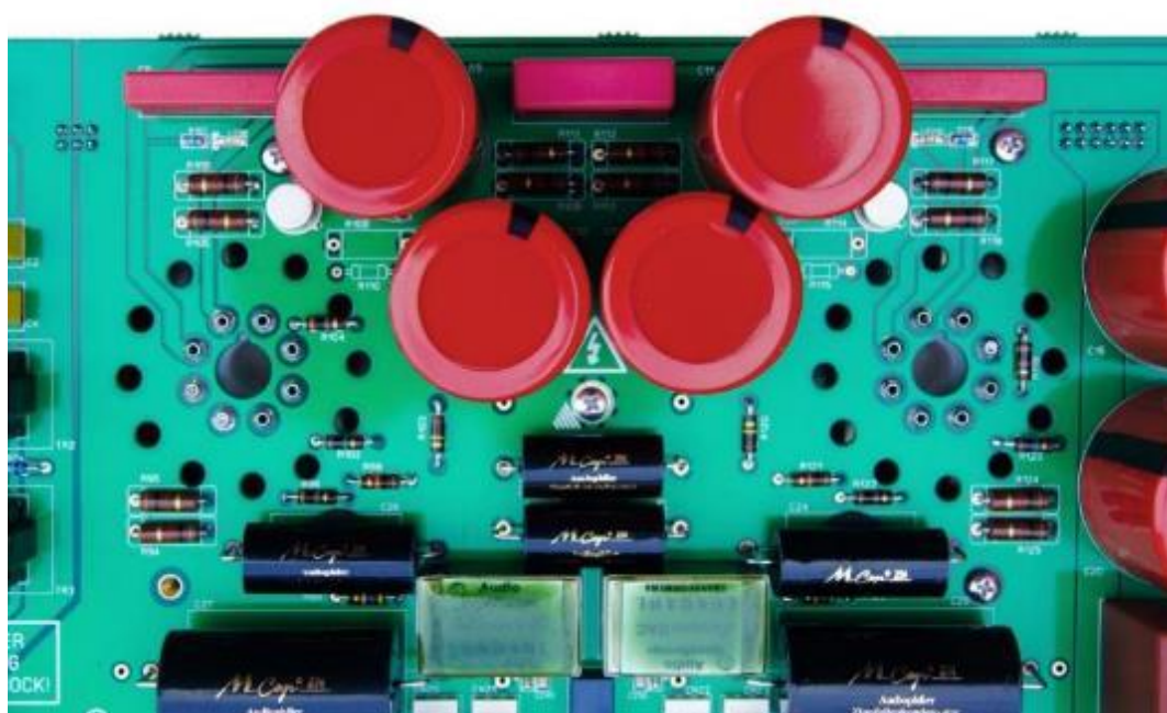
Fig. 6: The board for the tube Output Stage with the tubes sockets on the opposite side
